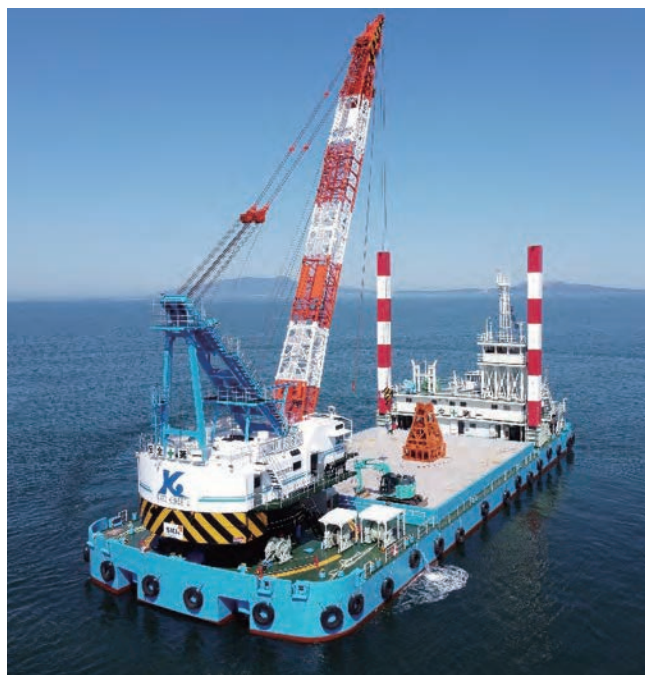
300t吊起重機船
