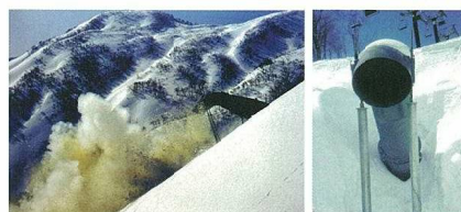
ガス砲 スキー場では事前に人工雪崩を発生させ予想される雪崩災害を軽減します。(新潟県妙高市) Gas Explosions(Gaz.ex) In order to reduce the effects of potential avalanches, before they occur naturally, gas explosions are used to artificially start avalanches. (Myokoh City, Niigata Pref.)
