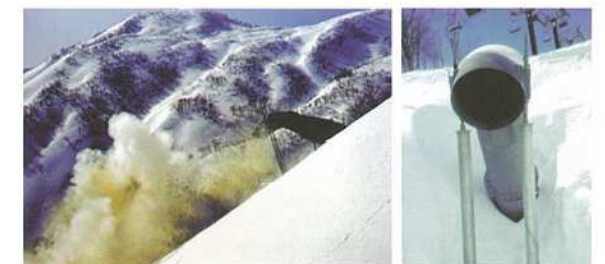
ガス砲 スキー場では事前に人工雪崩を発生させ予想される雪崩災害を軽減します。(新潟県妙高市) Gas Explosions(Gaz.ex) In order to reduce the effects of potential avalanches, before they occur naturally, gas explosions are used to artificially start avalanches. (Myokoh City, Niigata Pref.)
